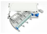
MFPS Fiber Optic panel, 1RU, 96 fibers/RU, splice/patch, SMOUV/front patch cords orientation to the right, 96 LC/UPC, OM4
