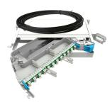
MFPS Fiber Optic panel, 1RU, 48 fibers/RU, pre-cabled I/O LSZH, 100m, front patch cords orientation to the right, 48 LC/APC, grade C
