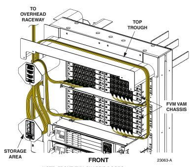
NOTE: FRONT FVM CHASSIS DOORS AND REAR NG3 CABLE MANAGEMENT ARE NOT SHOWN FOR CLARITY.
