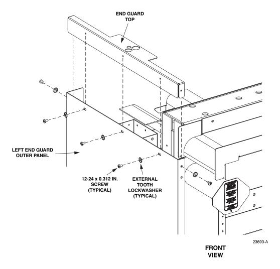
Figure 9. Assembling the End Guard Top to the End Guard
