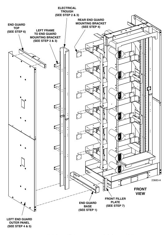
Figure 1. Left Side Installation on Frame Exploded View and Steps
