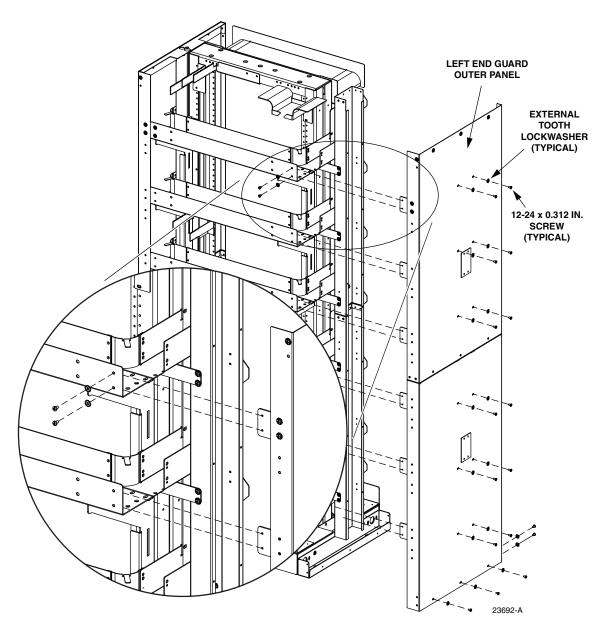
Figure 8. Assembling the End Guard to the Frame
