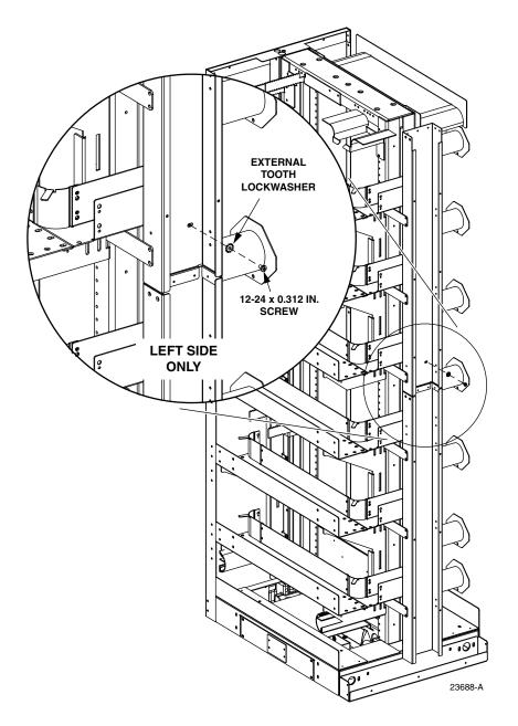
Figure 6. Securing Left Side Electrical Trough
