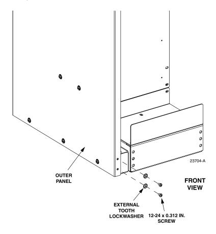
Figure 20. Attaching End Guard Bottom
