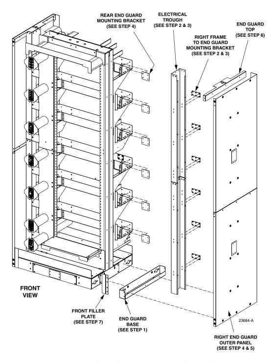
Figure 2. Right Side Installation on Frame Exploded View and Steps
