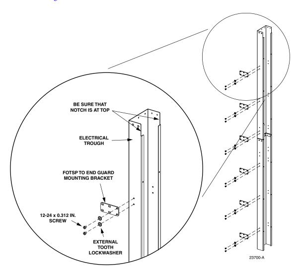
Figure 15. Installing Mounting Brackets on Electrical Trough
