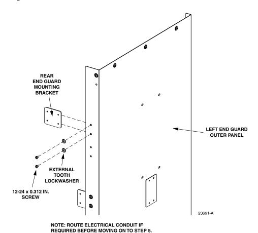
Figure 17. Installing the Rear End Guard Mounting Brackets
