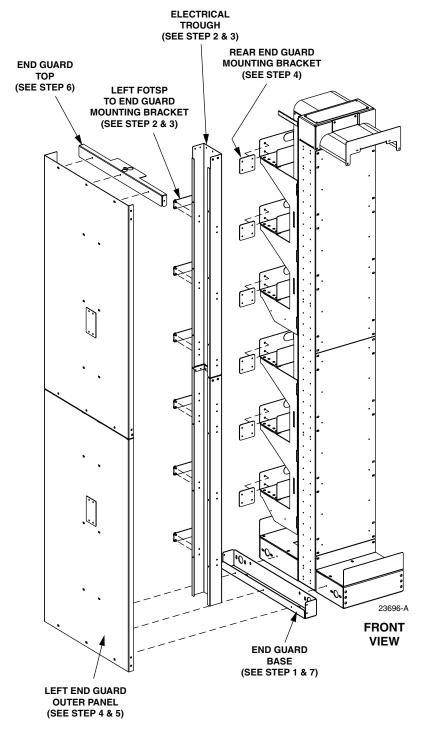
Figure 12. Left Side Installation on FOTSP Exploded View and Steps
