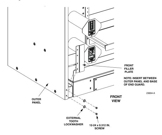
Figure 10. Installing the Front Filler Plate to the End Guard
