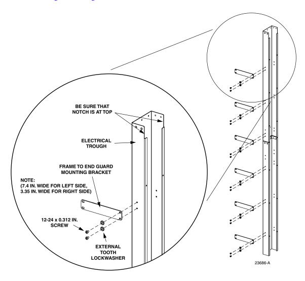
Figure 4. Installing End Guard Mounting Brackets on Vertical Trough
