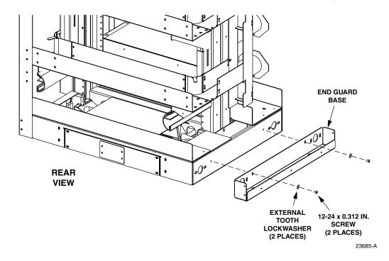
Figure 3. Assembling End Guard Base to Base of Frame
