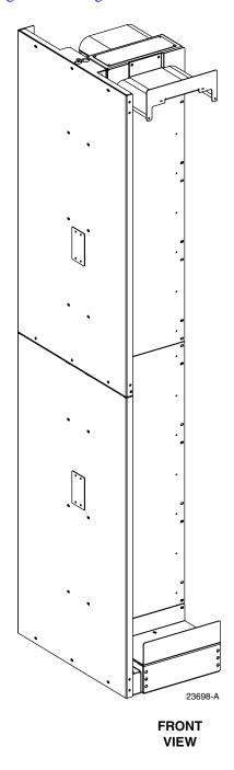
Figure 21. End Guard Installed on FOTSP
