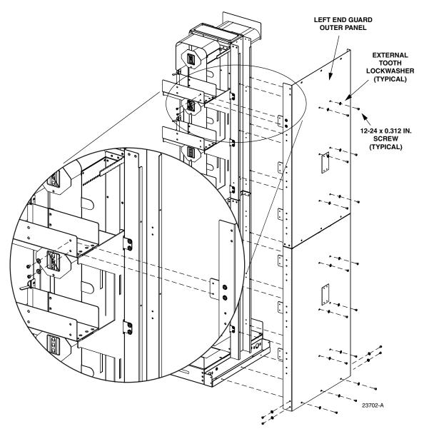
Figure 18. Assembling End Guard on FOTSP
