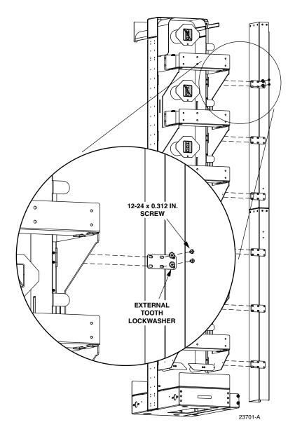
Figure 16. Assembling Electrical Trough on FOTSP
