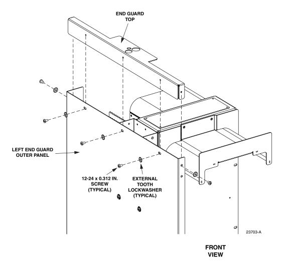
Figure 19. Installing End Guard Top on End Guard
