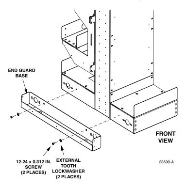
Figure 14. Installing the End Guard Base on the FOTSP
