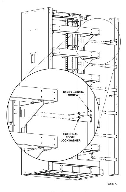
Figure 5. Assembling Electrical Trough to Frame
