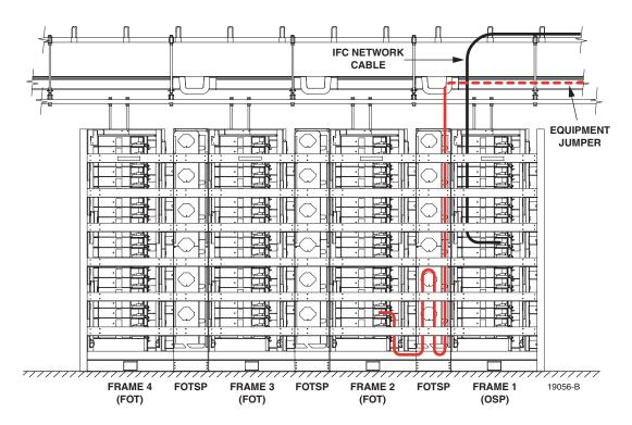
Figure 22. Cross-Connect With FOTSP's - Rear View
