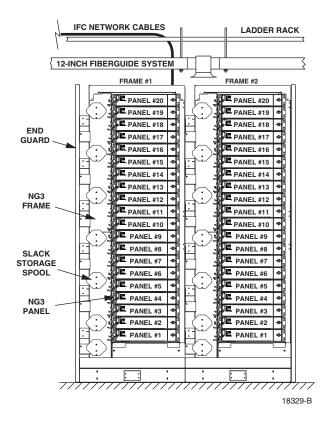
Figure 1. Typical NG3 High-Density Fiber Distribution Frame System
