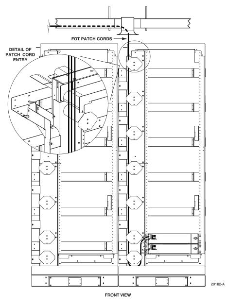
Figure 18. Typical FOT Patch Cord Overhead Routing - Interconnect Application
