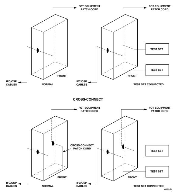
Figure 26. Series Test Access
