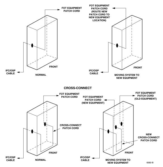
Figure 28. Moving Optical Fiber to New Equipment
