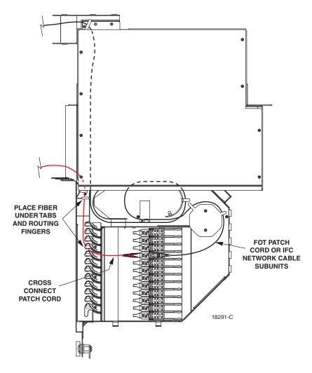
Figure 29. Patch Cord Routing Within Panel
