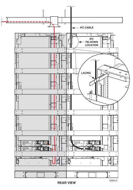
Figure 17. Typical IFC Cable Overhead Routing - All Applications
