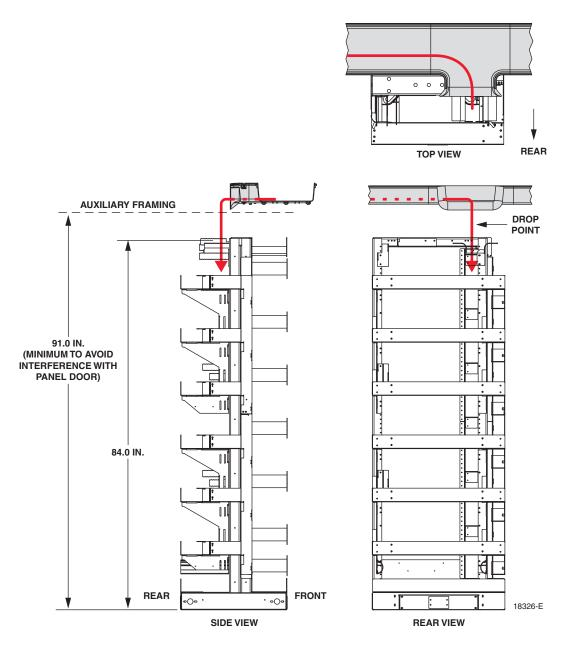
Figure 21. FiberGuide Placement for Cross-Connect Application
