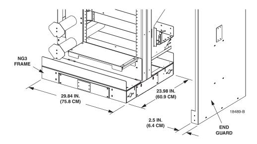
Figure 16. Dimensions of Single Frame and End Guard
