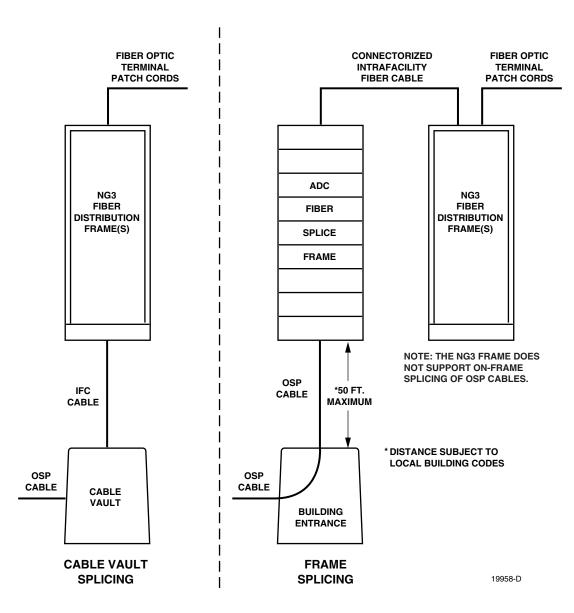
Figure 12. Cable Vault vs. On-Frame Splicing
