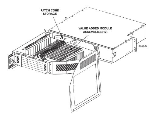
adapter ports. The same adapter types offered with the termination panel and termination/splice panel are also available with the VAM assembly.
