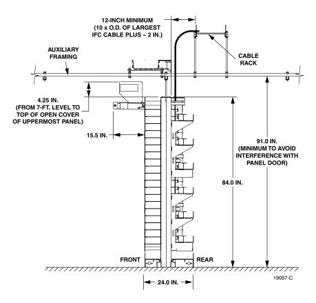
Figure 24. Cross-Connect With FOTSP's (Side View)
