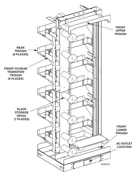
Figure 2. NG3 High Density Distribution Frame Main Components
