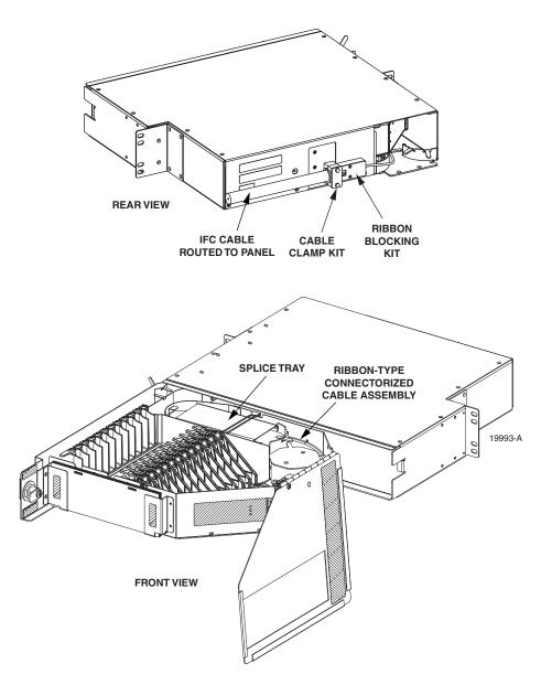
Figure 5. NG3 72-Position Termination and Splice Panel
