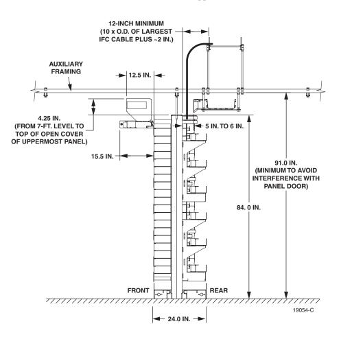
Figure 25. Alternative Placement of FiberGuide Raceway (Offset to Rear Rather Than Front Side)
