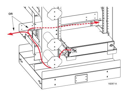
Figure 31. Path Cord Route Into Rear Trough
