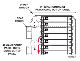
Figure 30. Typical Routing on Top Half of Frame
