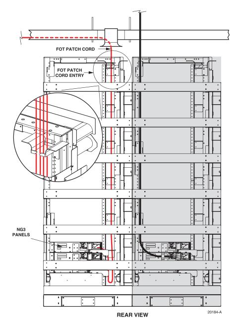
Figure 19. Typical FOT Patch Cord Routing - Cross-Connect Application
