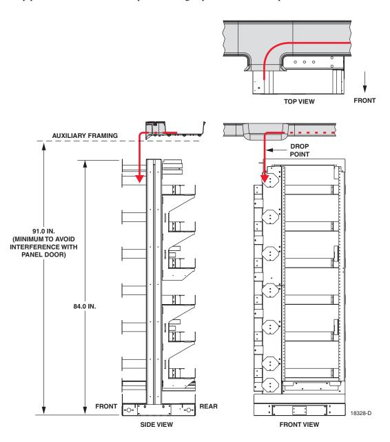
Figure 20. FiberGuide Placement for Interconnect Application
