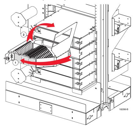
3. Locate the adapter pack to be connected and swing up the adapter pack to gain access to the adapters.
