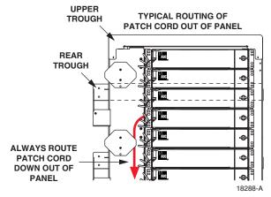
6. When using the rear trough, route the patch cord down and around the assigned slack storage spool (refer to next page), then route the patch cord through the rear trough as shown.
