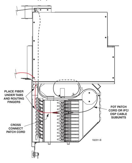
5. Swing the panel closed and route the patch cord down out of the panel as shown. For routing direction beyond the arrow, refer to the appropriate routing diagram in this guide.
