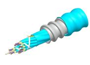
Fiber indoor cable, Riser/LSZH rated, MPO Trunk, interlocking aluminum armored, OM4 multi-mode, 192 fiber, Feet jacket marking, Aqua jacket color, B2ca flame rating
