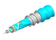
Fiber indoor cable, Plenum MPO Trunk, interlocking aluminum armored with plenum jacket, 48 fiber multi-unit with 16 fiber subunits, Gel-free, OM4 multi-mode, Feet jacket marking, Aqua jacket color
