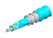
Fiber indoor cable, Plenum MPO Trunk, interlocking aluminum armored with plenum jacket, 144 fiber multi-unit with 16 fiber subunits, Gel-free, OM4 multi-mode, Feet jacket marking, Aqua jacket color
