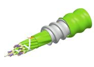
Fiber indoor cable, Riser/LSZH rated, MPO Trunk, interlocking aluminum armored, OM5 multi-mode, 16 fiber, Feet jacket marking, Lime green jacket color, B2ca flame rating
