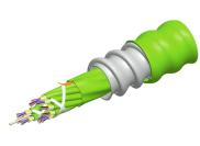
Fiber indoor cable, Plenum MPO Trunk, interlocking aluminum armored with plenum jacket, 144 fiber multi-unit with 16 fiber subunits, Gel-free, OM5 multi-mode, Feet jacket marking, Lime green jacket color
