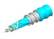
Fiber indoor cable, LazrSPEED® Riser/LSZH rated, MPO Trunk, interlocking aluminum armored, Multimode OM4, 8 fiber, Gel-free, Feet jacket marking, Aqua jacket color, B2ca flame rating
