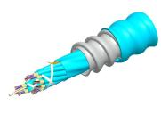
Fiber indoor cable, LazrSPEED® Riser/LSZH rated, MPO Trunk, interlocking aluminum armored, Multimode OM4, 24 fiber, Gel-free, Feet jacket marking, Aqua jacket color, B2ca flame rating
