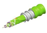
Fiber indoor cable, Low Smoke Zero Halogen Riser MPO Trunk, interlocking aluminum armored with low smoke zero halogen riser jacket, Multimode OM5, 16 fiber, Gel-free, Feet jacket marking, Lime green jacket color, B2ca flame rating
