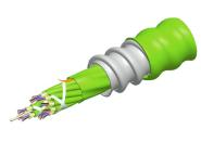
Fiber indoor cable, Riser/LSZH rated, MPO Trunk, interlocking aluminum armored, Multimode OM5, 64 fiber, Gel-free, Feet jacket marking, Lime green jacket color, B2ca flame rating
