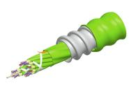
Fiber indoor cable, Riser/LSZH rated, MPO Trunk, interlocking aluminum armored, Multimode OM5, 192 fiber multi-unit with 8 fiber subunits, Gelfree, Feet jacket marking, Lime green jacket color, B2ca flame rating
