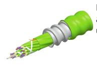
Fiber indoor cable, LazrSPEED® Plenum MPO Trunk, interlocking aluminum armored with plenum jacket, Multimode OM5, 48 fiber multiunit with 8 fiber subunits, Lime-green jacket color, Feet cable marking
