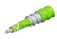
Fiber indoor cable, LazrSPEED® Plenum MPO Trunk, interlocking aluminum armored with plenum jacket, Multimode OM5, 192 fiber multiunit with 8 fiber subunits, gel-free, Feet jacket marking, Lime-green jacket color
