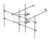
G23RHDX Tower Sector Frame with spine extension for RRU Mounting, 12.5 ft x 2.88 in OD face pipes, includes three 2.88 OD x 126 in antenna pipes
