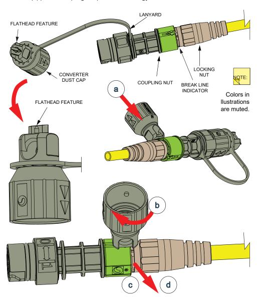
Remove the female converter from the Prodigy connector as follows:
