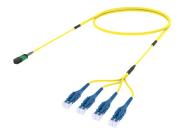
Singlemode MPO8 APC pinned to LC/UPC Uniboot Ruggedized fanout Cable, 8-Fiber, LSZH, 8 fiber PmP 2.0 mm /B2ca
