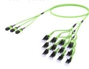
Ultra Low Loss ULL OM5 MPO8 UPC non-pinned to LC/UPC Uniboot Ruggedized fanout Cable, 24-Fiber, Plenum, 8 fiber PmP 2.0 mm
