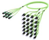
Ultra Low Loss ULL OM5 MPO8 APC pinned to LC/UPC Uniboot Ruggedized fanout Cable, 48-Fiber, Plenum, 8 fiber PmP 2.0 mm
