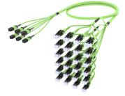
Ultra Low Loss ULL OM5 MPO8 UPC non-pinned to LC/UPC Uniboot Ruggedized fanout Cable, 48-Fiber, Dual Rated (OFNR/LSZH), 8 fiber PmP 2.0 mm
