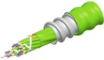
Fiber indoor cable, LazrSPEED® Plenum MPO Trunk, interlocking aluminum armored with plenum jacket, Multimode OM5, 72 fiber multi-unit with 12 fiber subunits, Lime-green jacket color, Feet cable marking
