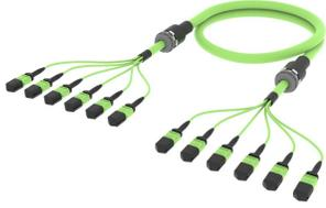
Ultra Low Loss (ULL) OM5 MPO12 UPC (pinned) to MPO12 UPC (pinned) Fiber Trunk Cable Assembly, 72-Fiber, Armored Indoor Plenum
