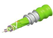
Fiber indoor cable, LazrSPEED® Riser/LSZH rated, MPO Trunk, interlocking aluminum armored, Multimode OM5, 192 fiber multi-unit with 12 fiber subunits, Feet jacket marking, Lime-green jacket color, B2ca flame rating
