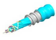
Fiber indoor cable, LazrSPEED® Riser/LSZH rated, MPO Trunk, interlocking aluminum armored, Multimode OM4, 288 fiber multi-unit with 12 fiber subunits, Gel-free, Feet jacket marking, Aqua jacket color, B2ca flame rating
