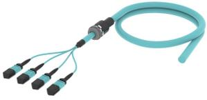
Ultra Low Loss (ULL) OM4 MPO12 UPC (pinned) to Unconnectorized Fiber Trunk Cable Assembly, 48-Fiber, Armored Indoor Dual Rated (OFNR /LSZH)
