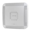
Carrier Access Point with MIMO 2x2 Radio Module for Low Power DCS 1800, IMT 2100 and TDD 3500 Applications, Fiber fed, DC
