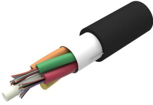
Fiber Indoor/outdoor Cable, Low Smoke Zero Halogen / 48 fiber Microsheath,, Gel-free, Singlemode , Meters jacket marking, Black jacket color, B2ca flame rating
