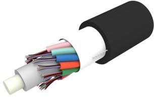
Fiber indoor/outdoor cable, LightScope® ZWP Low Smoke Zero Halogen, 144 fiber Microsheath, Singlemode, Gel-free, Meters jacket marking, Black jacket color, B2ca flame rating
