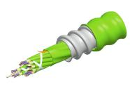
Fiber indoor cable, LazrSPEED® Plenum MPO Trunk, interlocking aluminum armored with plenum jacket, 48 fiber with 24-fiber, 3.0mm subunits, Gel-free, Multimode OM5, Feet jacket marking, Lime green jacket color
