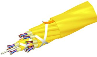
Fiber indoor cable, Plenum MPO Trunk, 24 fiber multi-unit with 8 fiber subunits, Singlemode G.657.A2, Feet jacket marking, Yellow jacket color
