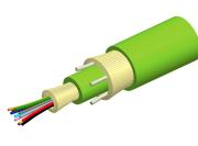
Fiber indoor cable, LazrSPEED® Low Smoke Zero Halogen MPO Trunk with 2.0mm Subunits, 12 fiber, Multimode OM5, Gel-free, Feet jacket marking, Lime green jacket color, B2ca Flame rating
