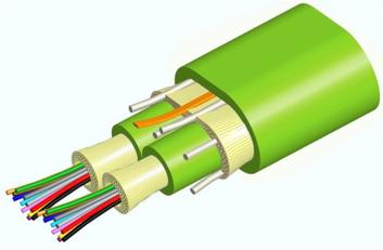
Fiber indoor cable, LazrSPEED® Low Smoke Zero Halogen Riser MPO Trunk, 24 fiber with 12 fiber 2.0mm subunits, Gel-free, Multimode OM5, Feet jacket marking, Lime green jacket color, B2ca flame rating
