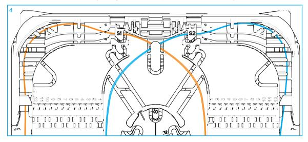
4 Overview of feeder fibers and branch fibers entering the top tray.
