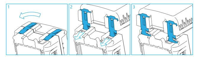
**Note:** If the hinges are installed in the top position, the cover **cannot be secured in open position**. To access the inside of the closure, the cover should be detached.
