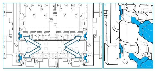
1 The 4 snap hooks at the bottom position can be released with a small screw driver.
