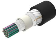
Fiber indoor/outdoor cable, All-Dielectric, LSZH Riser-Rated, Gel-Free, Central Tube Rollable Ribbon, 144 fiber, Singlemode G.657.A2/B2, Feet jacket marking, Black jacket color, Cca flame rating
