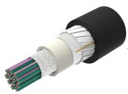
Fiber indoor/outdoor cable, All-Dielectric, LSZH Riser-Rated, Gel-Free, Central Tube Rollable Ribbon, 288 fiber, 200um Singlemode G.657.A2/B2, Feet jacket marking, Black jacket color, Cca flame rating
