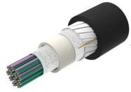
Fiber indoor/outdoor cable, All-Dielectric, LSZH Riser-Rated, Gel-Free, Central Tube Rollable Ribbon, 288 fiber, 200um Singlemode G.657.A2 /B2, Feet jacket marking, Black jacket color, Cca flame rating
