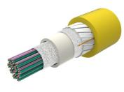
Fiber indoor cable, All-Dielectric, LSZH/Riser-Rated, Gel-Free, Central Tube 200µm Rollable Ribbon, 576 fiber, Singlemode G.657.A2/B2, Feet jacket marking, Yellow jacket color, Cca flame rating
