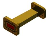
Taper Transition for WR112–WR137, 7.05–8.2 GHz, with interface types PDR84 and PDR70, 6 in, gray
