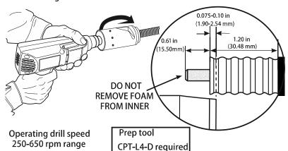
3 If all of the outer jacketing wasn't removed during initial cable prep remove at this time. Slide the clamping nut over the cable end. Install pre-lubricated o-ring in the 5th corrugation.
