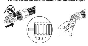
5 To achieve optimum Return Loss, pull outer body to remove coring bit from the tool. Place bit over inner conductor and push forward until bit contacts face of foam. BEFORE turning drill push HARD depressing foam. Maintaining force, turn drill at 1/4 trigger until tool bottoms out. Clean foam from coring bit and repeat, carefully remove any loose foam with non-metallic tool.
