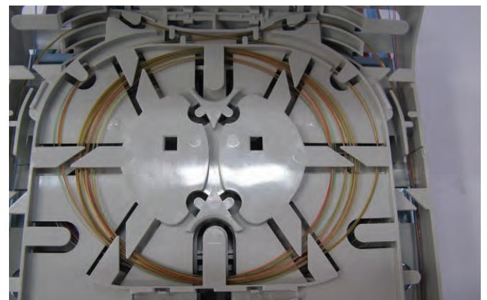
11.3.13 Route the fibers to the selected tray. See chapter 13 for detailed instructions concerning fiber routing.
