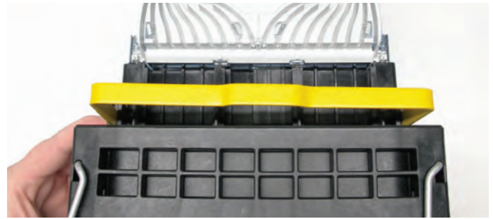
8.1.3 If cables are to be added, also the base should be removed. To remove the base, lift the yellow bracket that locks the base to the enclosure. The gel seal area will become accessible.
