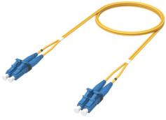
Fiber Optic Patch Cord, OS2, LC/LC duplex, 1.8 mm LSZH & OFNR, 32 m
