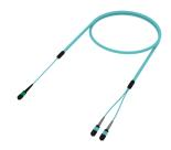
Ultra Low Loss OM4, 16F MM APC MPO (Unpinned) to 8F MPO (pinned), Fiber Extension Cable Assembly, 16-Fiber, Dual rate (LSZH/RISER)
