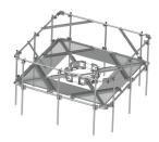
Four-sector HD Platform for 10" to 30" Monopoles, 14ft x 3.5" OD face pipes, 2.88" OD Top Rail, includes (12) 2.88" OD x 96" antenna pipes
