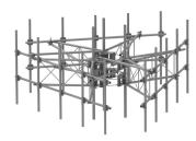
G23RHDXL PIM OPTIMIZED SPACING High Capacity Monopole platform with extended 10' Spine for RRU Mounting & extended frame for sites requiring increased sector to sector antenna spacing. 2 7/8in OD x 15ft face with (15) 2-7/8in OD x 96in Antenna pipes
