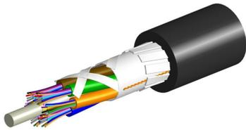
Fiber OSP cable, LightScope® ZWP Mini Single Jacket All-Dielectric, 24 fiber Arid Core construction, stranded loose tube, Gel-filled, Singlemode G.652.D and G.657.A1, Feet jacket marking, Black jacket color
