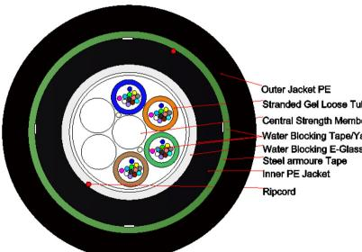
Stranded Gel Loose Tube Central Strength Member Water Blocking Tape/Yams Water Blocking E-Glass Yam
